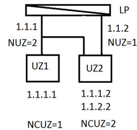
Figure 5. Example of a system with a circuit 1.1.1 supplying two different UZs (UZ1 and UZ2).
