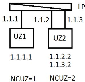
Figure 4. Example of UZ supplied from several circuits.
