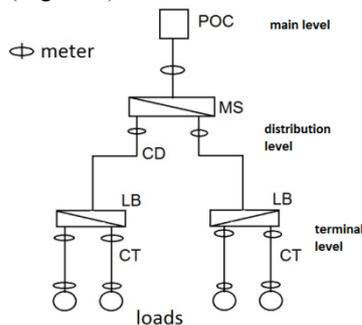
Figure 1. Example of power scheme
