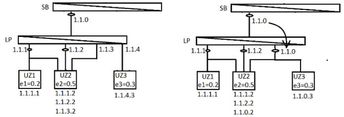
Figure 7. Level of coverage of a switchboard considering the upstream meter.
